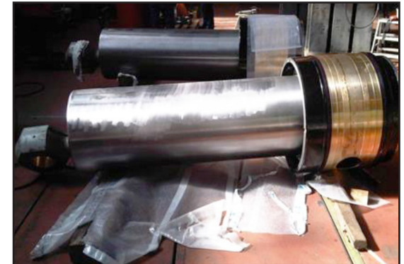
Servo motor rebuilt with Chesterton 22KE seal design made from AWC 800 polymer.
