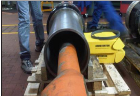
Servo motor cylinders being rebuilt.
